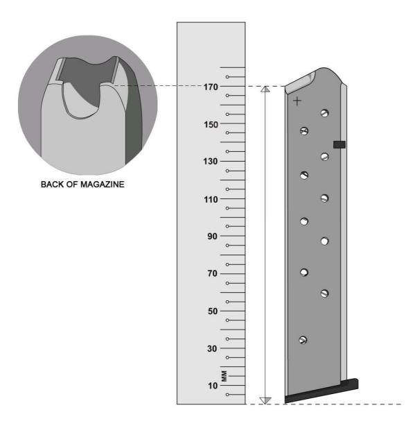
The magazine is placed vertically upright on a flat surface, with the measurement taken from the flat surface upwards to the rear of the feed-lips, as illustrated. Only straight, rigid magazines are permitted (i.e. flexible, drum, "J", "L", "T" or similar shape magazines are prohibited).
